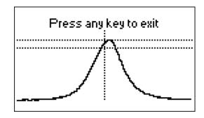
The top of the curve should be located in the middle of the screen, between the two horizontal dotted lines. A small horizontal shift of the curve is allowed. 0 – go to the third page of settings which contains reset commands.
