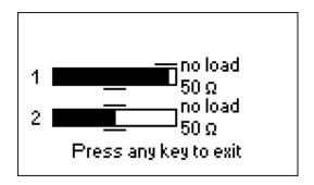
For the 50-Ohm load, the filled bars should stand at corresponding positions (notice the "no load" and "50  $\Omega$ " marks):
