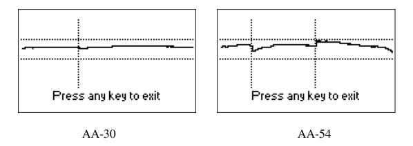
The voltage curve should stay between the horizontal dotted lines. The vertical lines are the bounds of analyzer's subbands.
